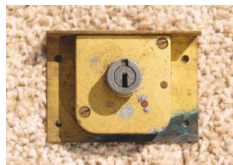
A tumbler lock similar to a Bramah lock
